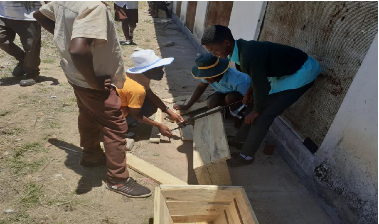
Picture above: Students using sash clamp to fix their hive
