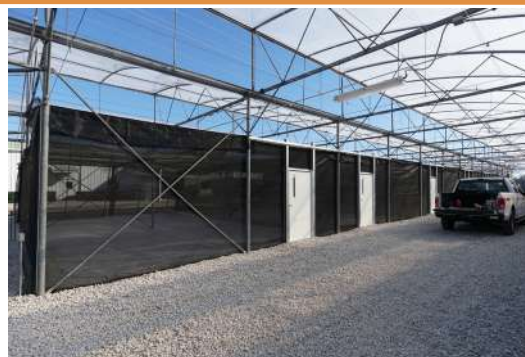
Figure 1. A view of the flight cages. Flight cages are fully enclosed and impermeable to insects as small as SHB. In total there are 12 individual cages, with six on either side of the gravel driveway, allowing for multiple assays to take place at once.
